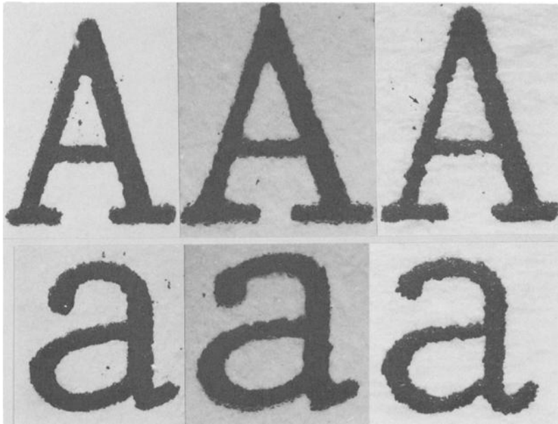
FIG. 10—Uppercase and lowercase "A's" for Prestige Elite elements for Royal 10/12 printwheel, on the left; Selectric III 96 character element, middle; and Smith Corona printwheel, right.
