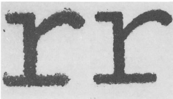
FIG. 2—Courier 10 lowercase “r” from a Selectric II element, on left, and Selectric III element, on the right.
